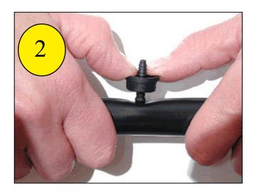
Push some Spaggetti tube onto the Output barb of the dripper
